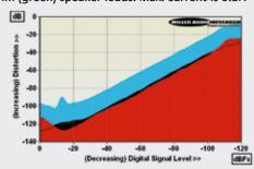
ABOVE: THD vs. digital level over a 120dB range at 1kHz (XM5 DAC, red; CD, black) and 20kHz (CD, blue)
