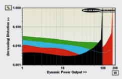
ABOVE: Dynamic power output versus distortion into 8ohm (black trace), 4ohm (red), 2ohm (blue) and 10hm (green) speaker loads. Max. current is 9.3A
